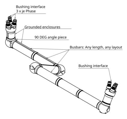
The key features for use in space are the robust, grounded aluminum enclosures with a quick assembly fitting design which allows fast and easy assembly and disassembly and full flexibility for transport to space. It uses the available vacuum as main insulation medium and requires a minimum number of insulators to withstand the high radiation in space.
